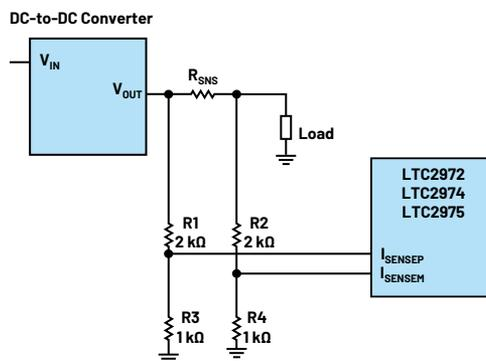
Figure 1. A resistor divider for current sense produces a large error.
