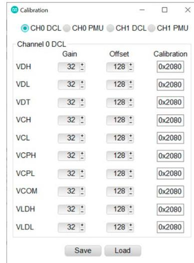
Figure 8. Calibration register setup for the MAX9979.
