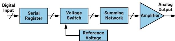
Figure 1. A digital-to-analog converter (DAC) block diagram.
