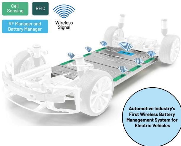
Figure 1. An electric vehicle using a wireless battery management system (wBMS).
