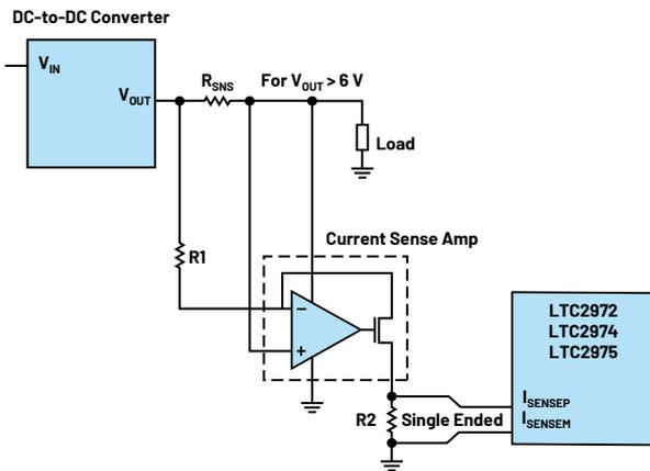
Figure 2. A current sense amplifier used as a level translator.
