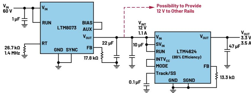
Figure 2. A circuit solution with the LTM8073 and LTM4624, downconverting 60 V input to 3.3 V output.
