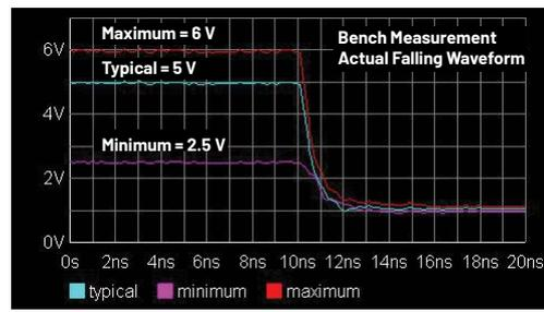
Figure 10. ADuM4146 FAULT pin falling waveform at VDD1 reference.
