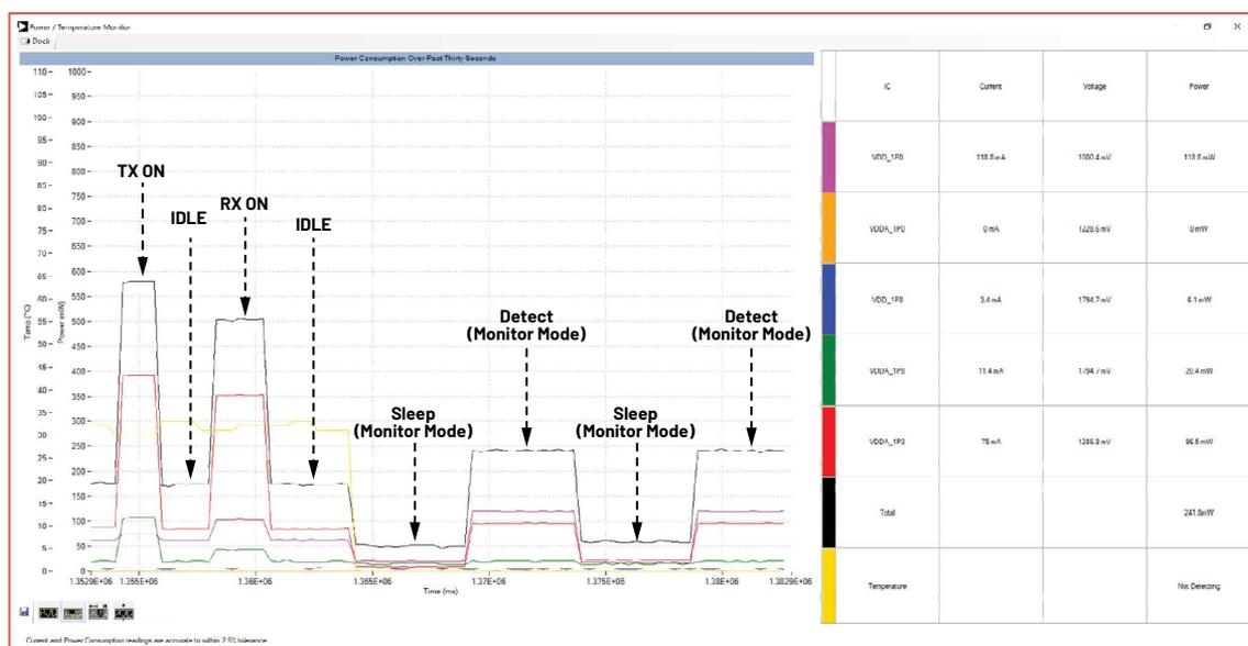
Figure 12. Power consumption real-time display using TES.
