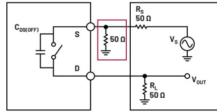
Figure 4. Off-isolation test circuit with a  $50 \Omega$  termination on the source.
