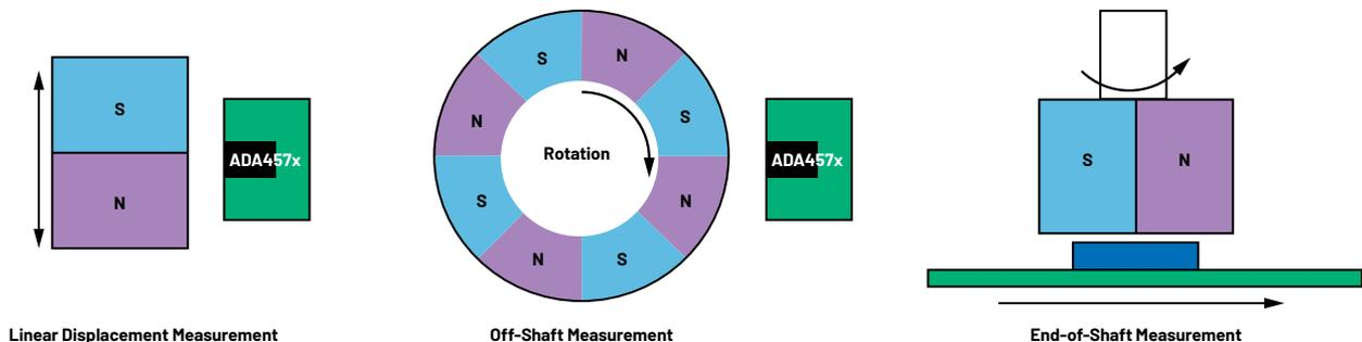
Figure 1. Linear displacement measurement (left), off-shaft measurement (middle), and end-of-shaft measurement (right).
