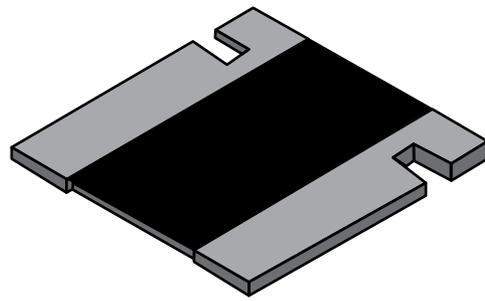
Figure 12. A 4-terminal shunt resistor.
