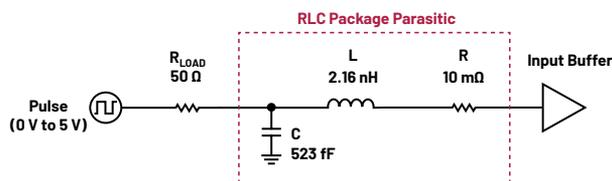
Figure 15. ADuM4146 transistor-level design simulation setup with loading conditions (input buffer).
