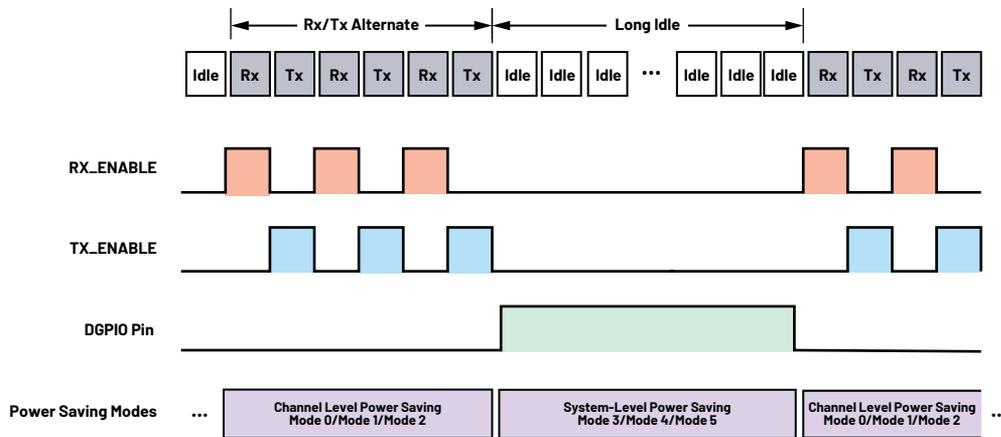
Figure 8. An example of using combined channel-level and system-level power saving.
