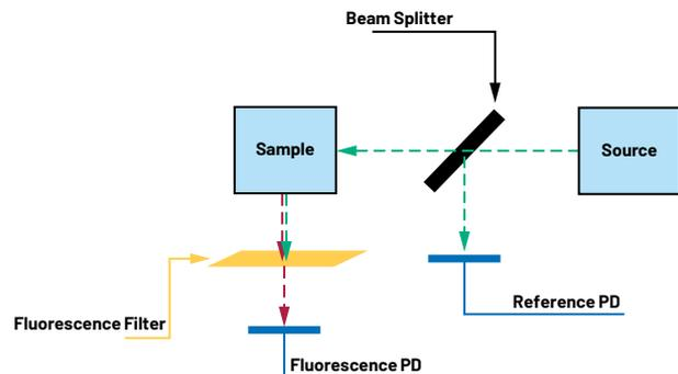
Figure 10. Optical path for fluorescence measurement.
