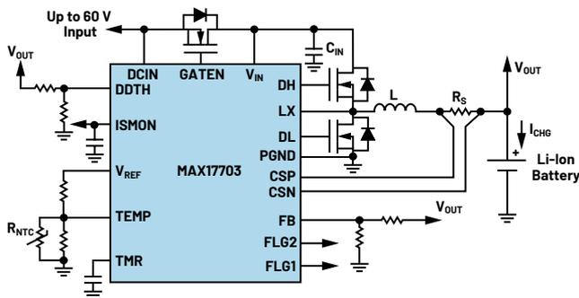
Figure 5. Advanced, high voltage Li-Ion battery charger circuit.
