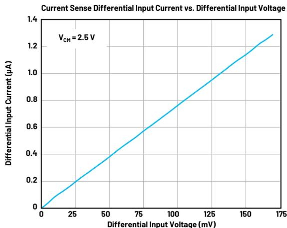
Figure 10.  $I_{SENSE}$  pin current.
