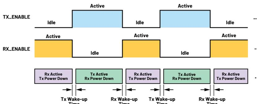
Figure 5. Channel-level power saving in a general TDD operation.
