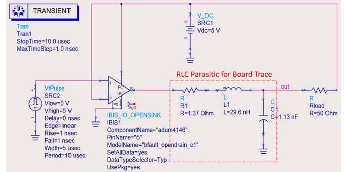
Figure 21. Actual IBIS simulation setup with loading conditions (open-drain buffer).
