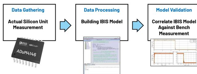
Figure 1. IBIS model through bench measurement generation process.
