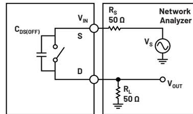
Figure 2. Off-isolation measurement test circuit.
