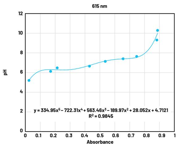
Figure 6. Absorbance calibration curve of pH at 615 nm.
