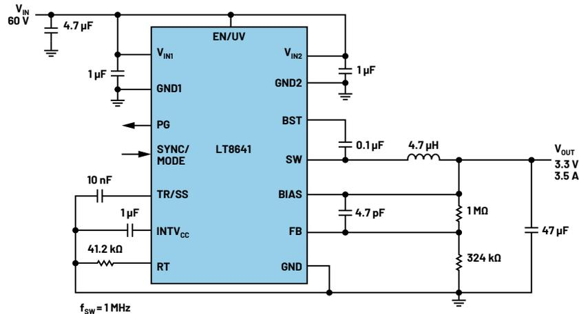
Figure 3. A circuit solution with the LT8641 downconverting 60 V input to 3.3 V output.
