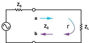
Figure 1. Transmission line with a matched signal source terminated in a single-port load.
