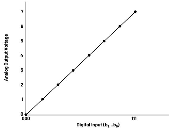
Figure 2. Ideal transfer function of a 3-bit DAC.
