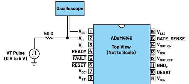
Figure 22. Bench setup with loading conditions (input buffer).
