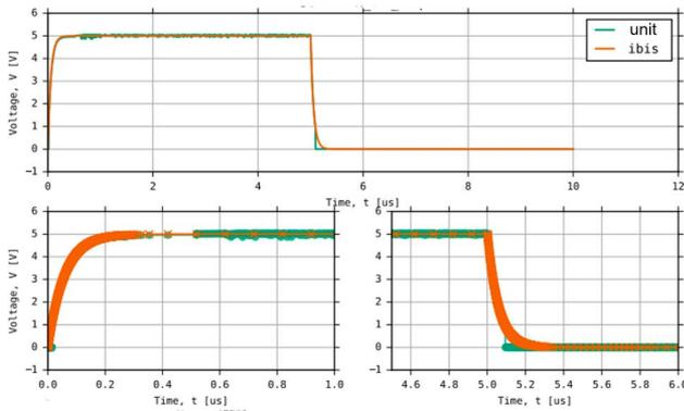
Figure 24. Actual silicon unit vs. IBIS model validation results (input buffer).
