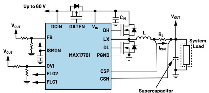
Figure 7. Supercapacitor high voltage, high current charger.
