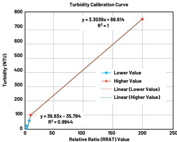
Figure 9. Calibration curve for turbidity.
