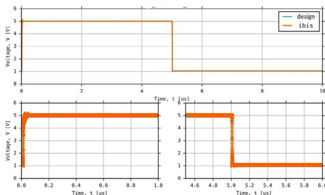
Figure 18. Transistor-level design vs. IBIS model validation results (open-drain buffer).
