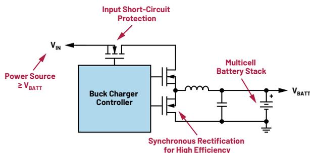
Figure 2. Generic synchronous rectification buck charger.
