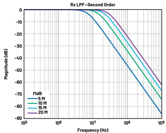
Figure 4. First-order and second-order Rx LPF frequency response at different LPF f1dB configurations.
