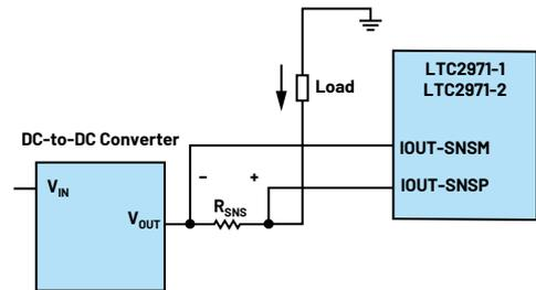
Figure 5. Sensing current on a negative rail without external components.
