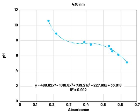
Figure 5. Absorbance calibration curve of pH at 430 nm.
