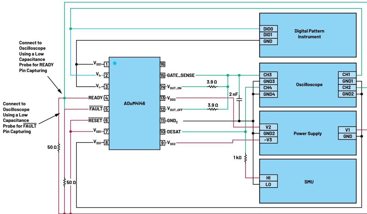
Figure 8. ADuM4146 bench setup for READY/FAULT switching behaviors.
