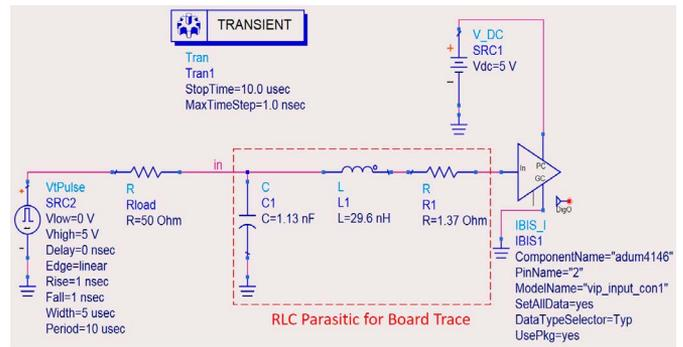
Figure 20. Actual IBIS simulation setup with loading conditions (input buffer).
