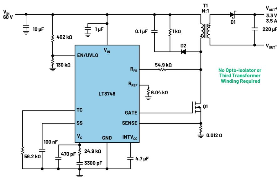
Figure 1. A circuit solution with the LT3748 downconverting 60 V input to 3.3 V output.
