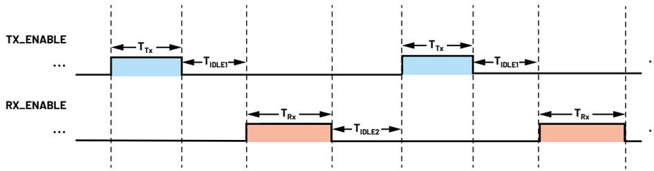
Figure 7. A general DMR TDD timing configuration for power consumption measurement using channel-level power saving modes.
