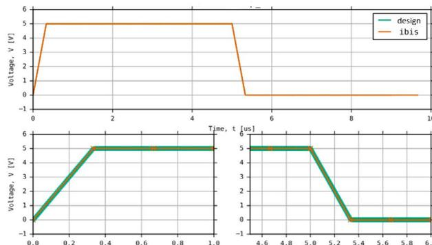
Figure 17. Transistor-level design vs. IBIS model validation results (input buffer).
