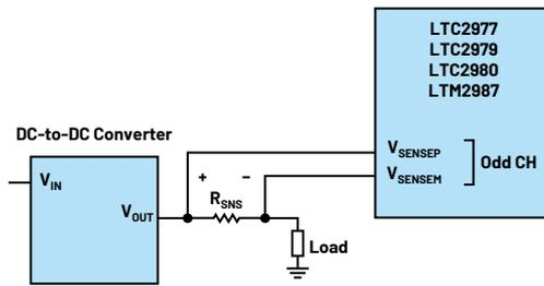
Figure 14. V<sub>SENSE</sub> pins used for differential current sensing.
