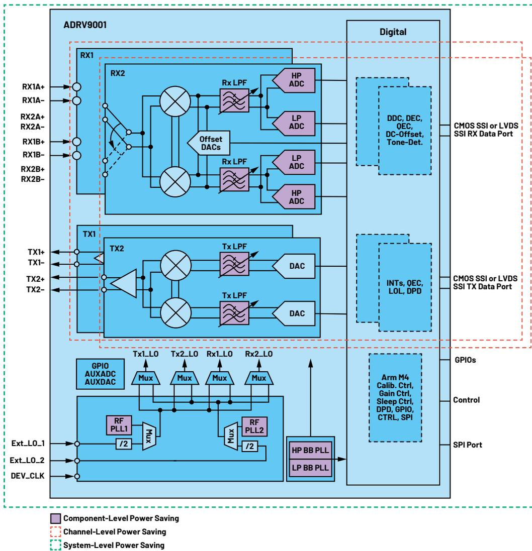
Figure 1. A high level diagram of the ADRV9001 power saving options at three different levels.
