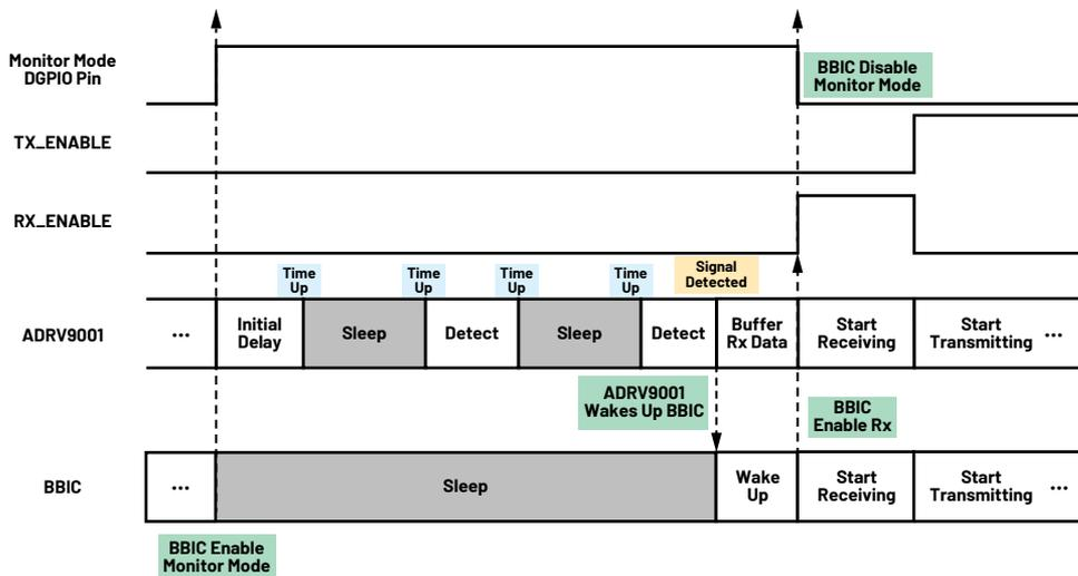
Figure 10. Timing events of ADRV9001 and BBIC during monitor mode.
