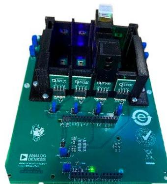
Figure 4. The CN0503 taking a pH measurement.
