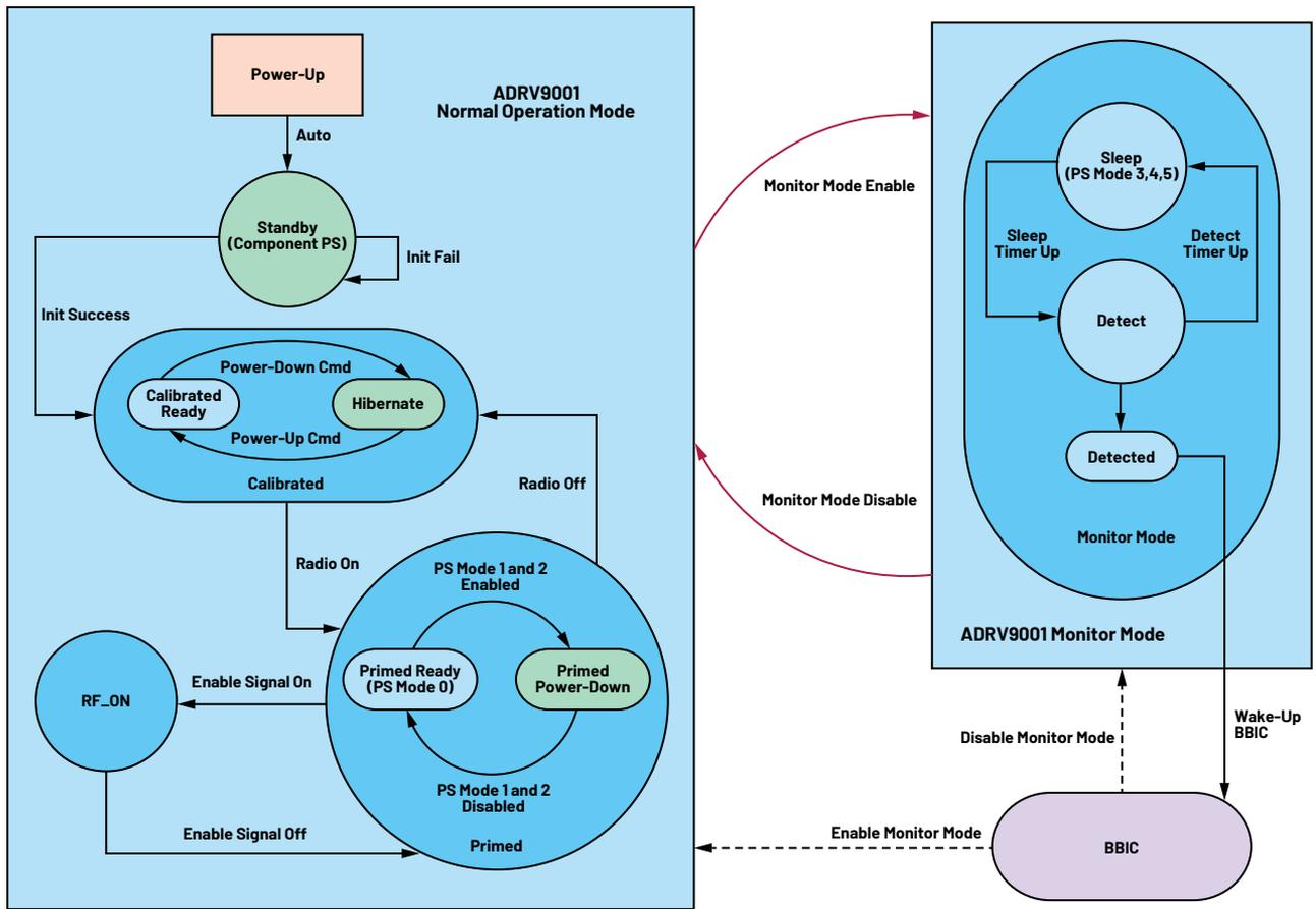
Figure 9. State diagram of the ADRV9001 in normal operation mode and monitor mode.
