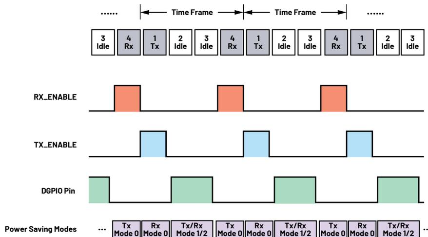
Figure 6. An example of using DGPIO to trigger channel-level power saving using Mode 1 or Mode 2.
