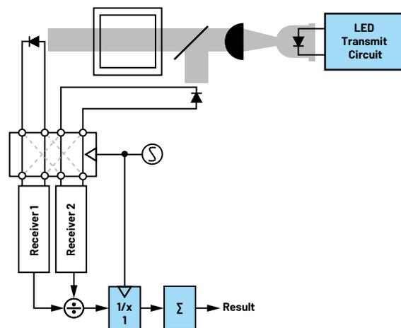
Figure 3. An optical light path for measuring absorbance.
