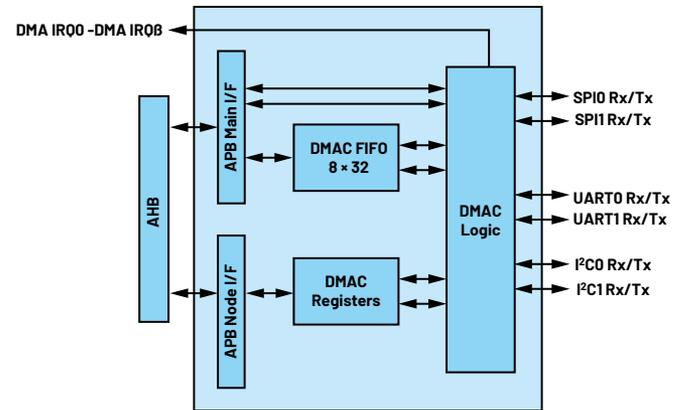
Figure 4. An architectural diagram of the DMA controller on the MAX32660.
