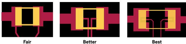
Figure 11. Layout proposals for shunt resistors.
