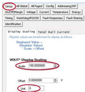
Figure 15. VOUT Display Scaling in the Setup tab.
