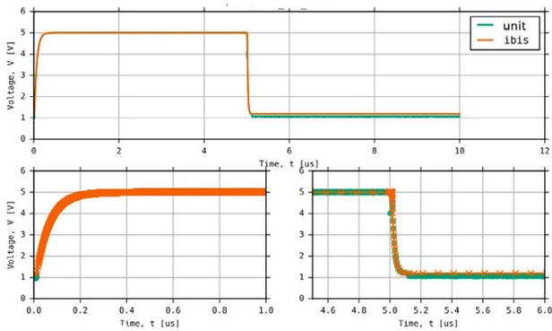
Figure 25. Actual silicon unit vs. IBIS model validation results (open-drain buffer).
