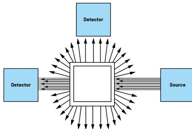
Figure 7. Optical path for turbidity measurement.
