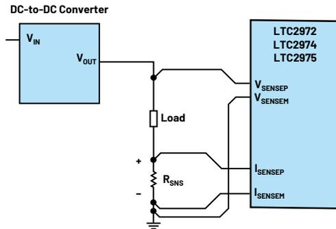
Figure 3. Low-side sensing solves high voltage current sensing but has drawbacks.
