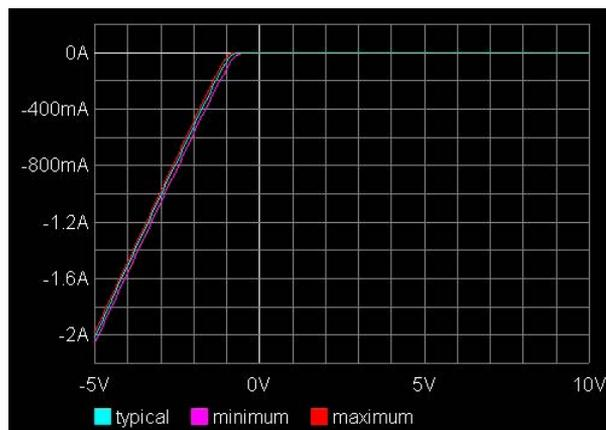
Figure 6. ADuM4146 input buffer bench measured ground clamp.
