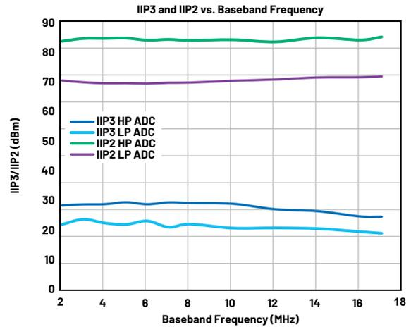
Figure 3. ADRV9001 linearity performance comparison between its HP ADC and its LP ADC.
