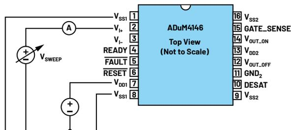
Figure 5. ADuM4146 bench setup for I-V clamp measurement.
