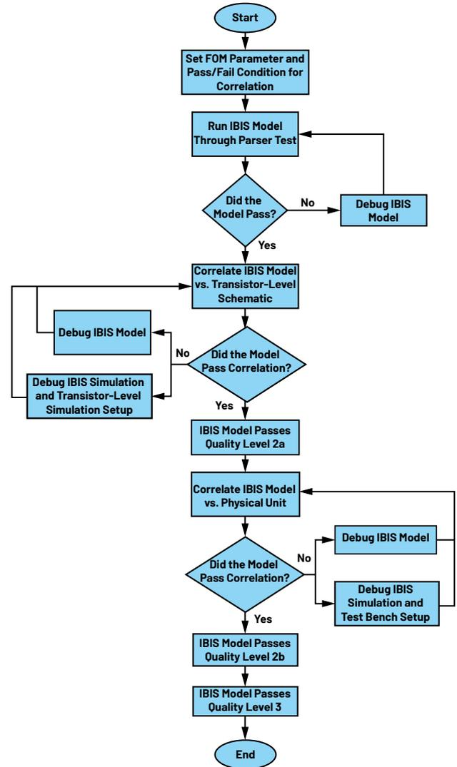
Figure 12. IBIS model Quality Level 3 validation process flowchart.
