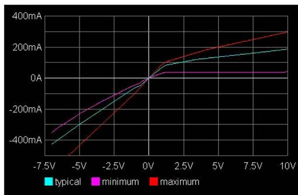
Figure 7. ADuM4146 open-drain buffer pull-down result.
