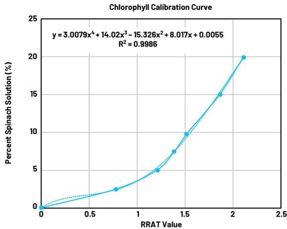
Figure 12. Calibration curve for percent spinach solution.
