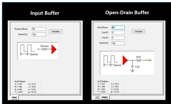
Figure 14. ADuM4146 input and open-drain buffer simulation setup.
