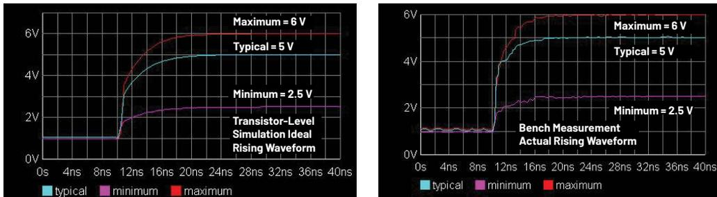
Figure 9. ADuM4146 FAULT pin rising waveform at VDD1 reference.
