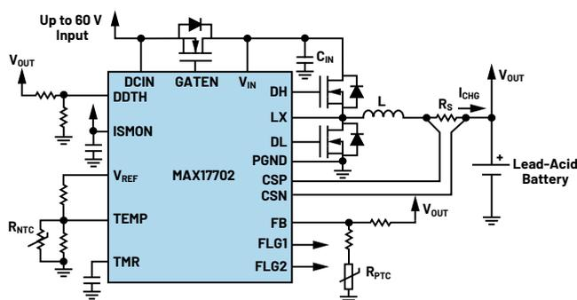
Figure 3. High voltage lead-acid battery charger controller.
