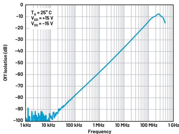
Figure 1. ADG5412 off isolation vs. frequency, ±15 V dual supply.
