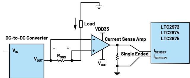
Figure 4. Sensing current with a CSA (LTC6105).
