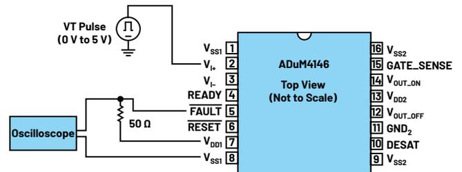
Figure 23. Bench setup with loading conditions (open-drain buffer).
