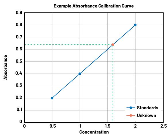
Figure 1. An example of a calibration curve for absorbance.
