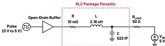
Figure 16. ADuM4146 transistor-level design simulation setup with loading conditions (open-drain buffer).
