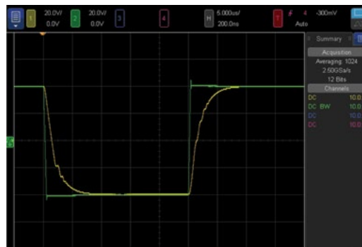
Figure 9. Large signal response to overloading input slew rate ( \pm 130 V/ \mu s).
