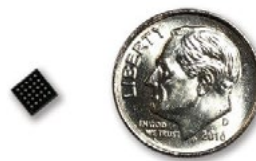
Figure 1. The LTM8074 uses Silent Switcher ® architecture for a complete low noise solution in a tiny package.
