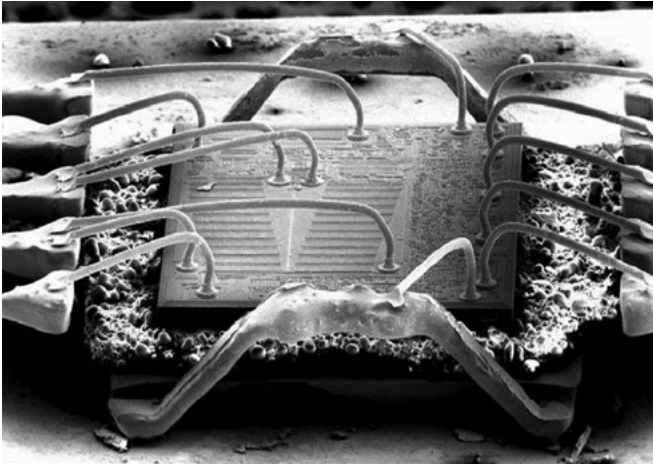
Figure 4. Wirebond shown in a disassembled LT8610.
