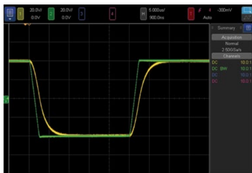
Figure 8. Large signal response to moderate input slew rate ( \pm 32 V/ \mu s.)
