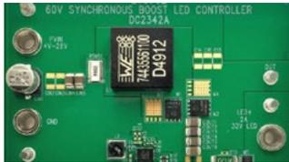
**31 Synchronous Boost Converter Powers High Current LEDs Even at Low Input Voltages**
