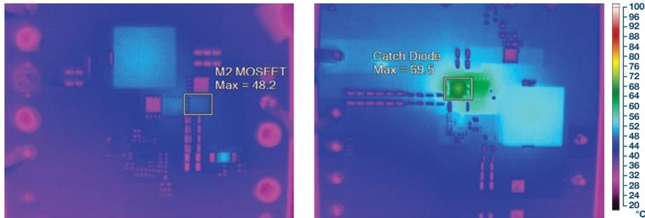
Figure 3. Under identical test conditions and using similar component selection, the synchronous LT3762 (left) powers a 32 V string of LEDs at 2 A with far less temperature rise than observed in an asynchronous LT3755-2 circuit (right). This increase in thermal performance is attributed to replacing the Schottky catch diode with a synchronous MOSFET, which eliminates the loss caused by the forward voltage drop of the diode.
