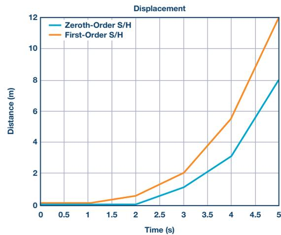
Figure 7. The comparison between zeroth-order and first-order integration methods in velocity calculation.
