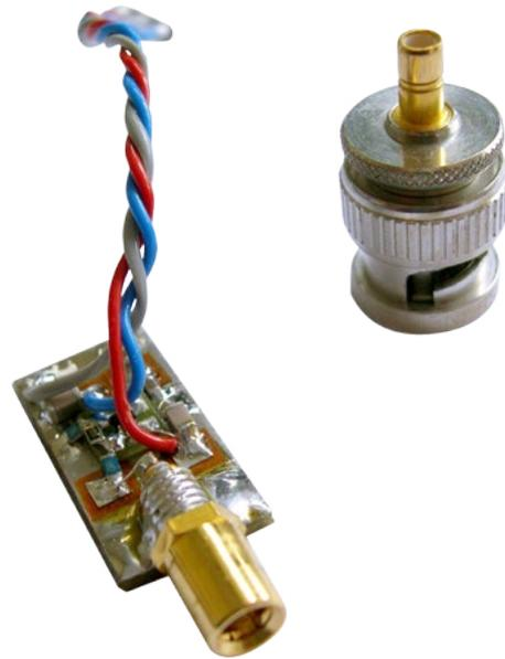
Figure 2. Prototype pocket-size white noise generator.
