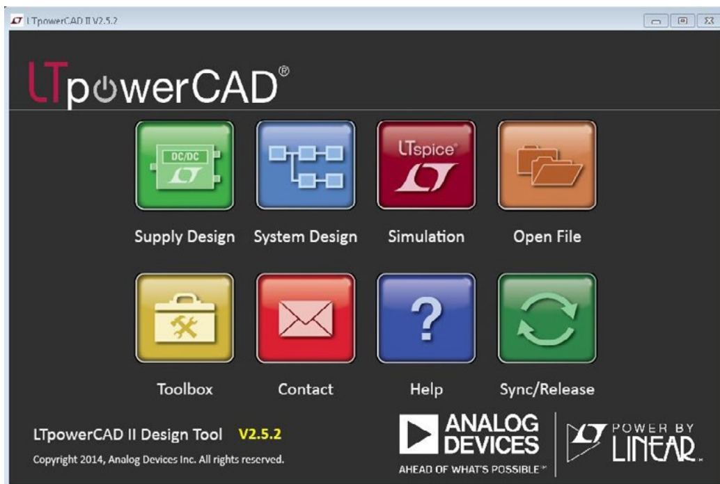
Figure 1. LTpowerCAD tool to select the right dc-to-dc converters to power FPGAs.
