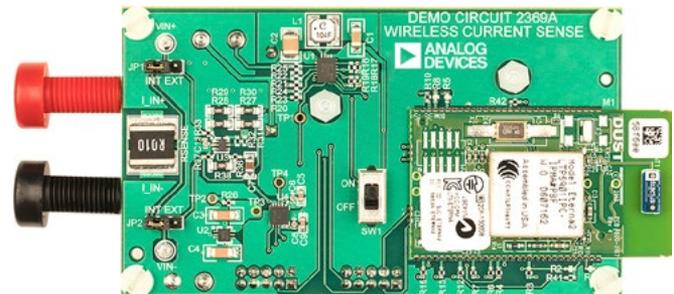
Figure 3. A complete wireless current sense circuit is implemented on a small PCB. The only physical connections are the banana jacks for the current to be measured. The wireless radio module is shown on the right. The circuit is powered from two AAA batteries connected on the back of the board.
