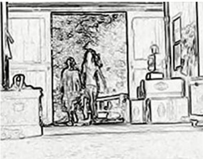
Figure 3. ADIS17002 logarithmic image exposure with built-in edge detection.
