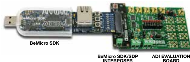
图6. BeMicro SDK/SDP转接板连接子板与BeMicro SDK
