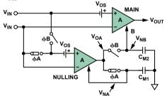
Figure 1. Phase A of auto-zero amplifier: nulling phase.
