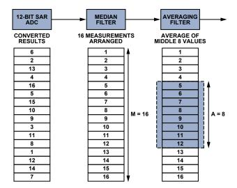
Figure 4. Median and average filtering.
