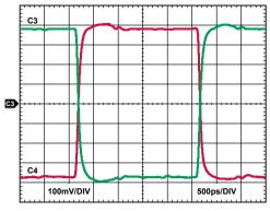
Figure 2. ADCLK954 clock buffer output waveforms with 3.3-V supply.
