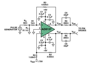
Figure 8. PIN-diode driver schematic.
