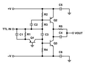
Figure 6. Discrete switch driver circuit.
