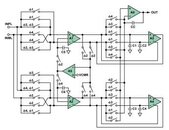
Figure 4. The AD8628 combines auto-zeroing with chopping to achieve wider bandwidth.
