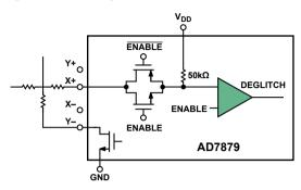
Figure 3. Wake-up-on-touch setup.
