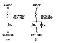
Figure 2. PIN diode equivalent circuits. a) On,  $I_{BIAS} >> 0$ . b) Off,  $V_{BIAS} \leq 0$ .
