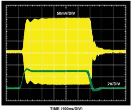
Figure 12. Waveform showing RF switching speed.
