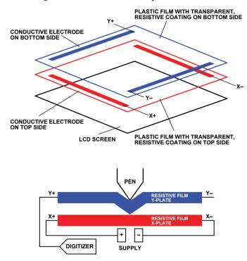
Figure 1. Construction of a resistive touch screen.
