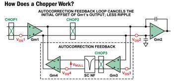
Figure 3. Chopping scheme used in the ADA4051.
