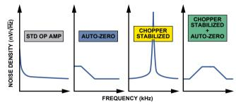
Figure 5. Typical noise of various amplifier topologies vs. frequency.
