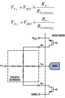
Figure 2. X-position measurement.
