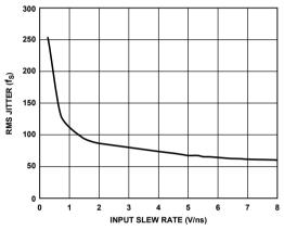
Figure 1. ADCLK925 rms jitter vs. input slew rate.
