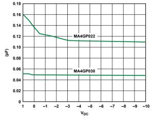
Figure 9. GaAs CT capacitance vs. voltage.
