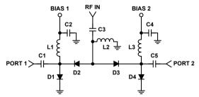
Figure 5. Typical single-pole, double-throw (SPDT) switch circuit.
