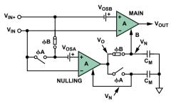
Figure 2. Phase B of auto-zero amplifier: auto-zero phase.
