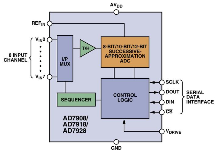
Figure 5. Functional block diagram of a modern 1-MSPS SAR ADC with 8-channel input multiplexer. Its family includes the AD7908<sup>5</sup> (8 bits), AD7918<sup>6</sup> (10 bits), and AD7928<sup>7</sup> (12 bits).
