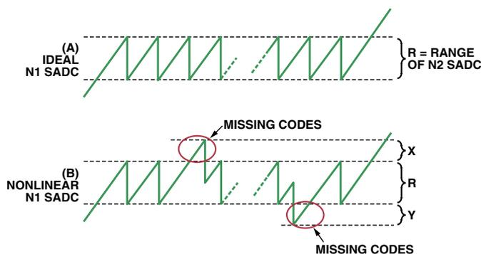
Figure 12. Residue waveform at input of second-stage SADC.
