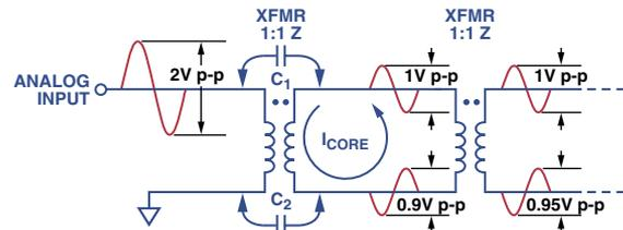
Figure 5. Two transformers in cascade improve signal balance.
