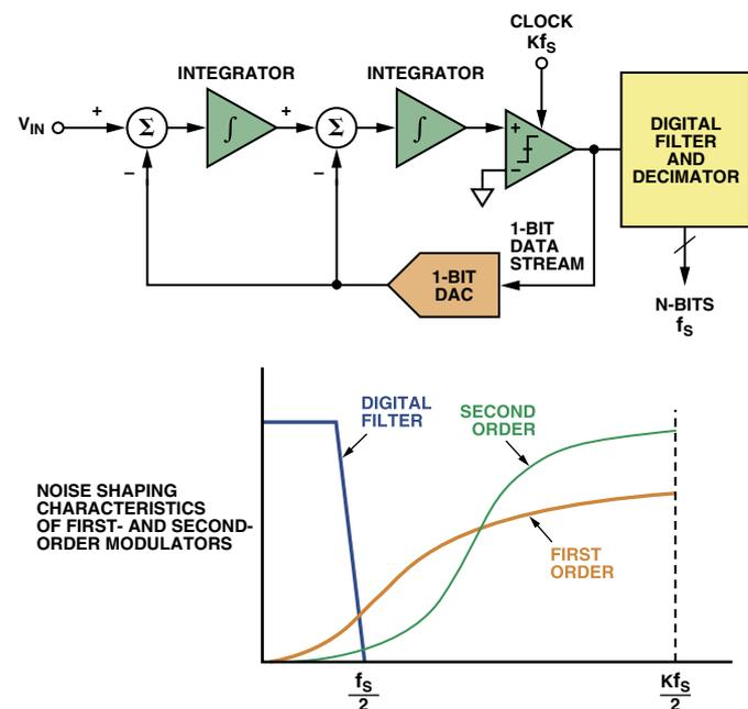
Figure 8. Second-order  $\Sigma$ - $\Delta$  modulator.
