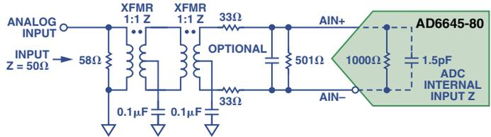
Figure 4. Cascaded transformers.
