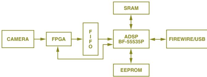
Figure 4. Block diagram of the processing board.
