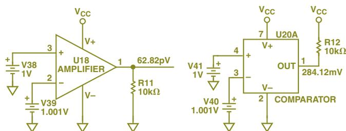
Figure 1. Responses of single-supply amplifier (63 pV) and comparator (280 mV) models to a  $-1\text{-mV}$  input-voltage difference.
