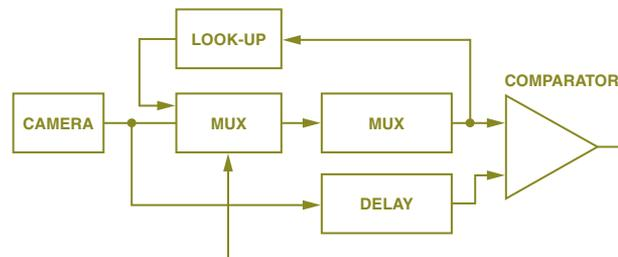
Figure 7. Simplified signal flow diagram of the 1D AR.
