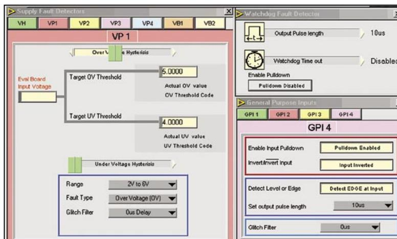
Figure 2. ADM1060 graphical user interface (GUI).
