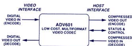
Figure 1. Basic functions of the ADV601.
