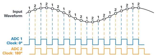
Figure 2. Two interleaved 100 MSPS ADCs—clocking and samples.
