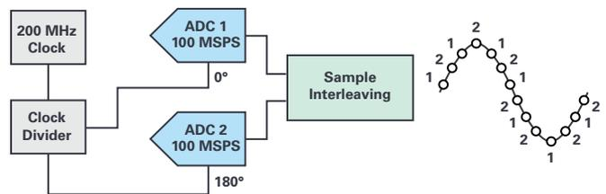
Figure 1. Two interleaved 100 MSPS ADCs—basic diagram.
