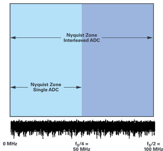
Figure 3. Two interleaved ADCs—Nyquist zone.
