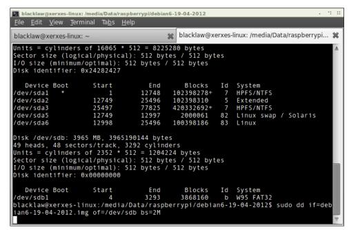
FIGURE 1-5: Flashing the SD card using the dd command in Linux
