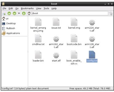
If you're having problems with graphics output, such as the image not filling the screen or spilling over the edge, config.txt is where you'll be able to fix it. Normally, the file is empty or—on some distributions—simply not present; this just means that the Pi will operate using its preset defaults. If you want to make changes and the file isn't there, just create a new text file called config.txt and fill in the settings you want to change.
