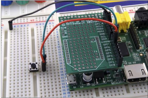
The connections for an XBee wireless interface could also prove useful if you are considering using the Pi in an embedded computing project. When combined with a compatible transceiver—such as an XBee, RF-BEE or RN-XV module—it allows for wireless access to the Pi's UART serial port. Such access could be used to read sensor details from the Pi, take control of the Pi's software or even control a Pi-powered robot from a remote location.
