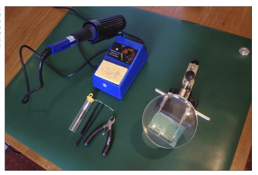
If you're doing delicate, close-up work, you should wear protective glasses. Sometimes the boiling flux inside the solder can cause it to spit upwards, and if it hits you in the eye, you'll be in for a world of pain.
