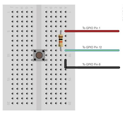
FIGURE 12-5: The example breadboard layout for a simple pushbutton input The circuit you just built creates a situation whereby the input pin, which in this instance is Pin 12 of the Raspberry Pi's GPIO port, is constantly *high* thanks to the pull-up resistor connected to a 3.3 V supply. When the push-button is pressed, the circuit is grounded and becomes *low*, providing the cue for your Python program to know that the button has been activated.
