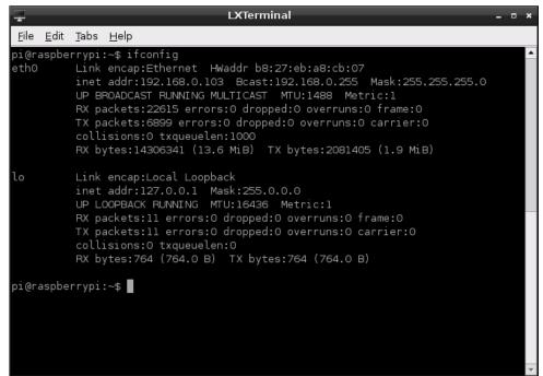
FIGURE 3-2: The output of ifconfig on a Raspberry Pi Model B
