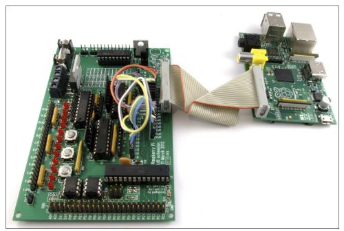
FIGURE 13-8: The Gertboard connected to a Raspberry Pi
