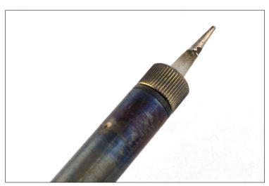
FIGURE 12-10: A soldering iron tip that is in the process of being tinned with solder
