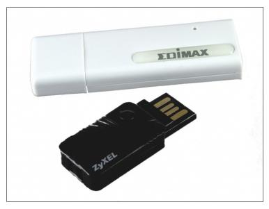
FIGURE 1-8: Two USB wireless adapters, suitable for use with the Raspberry Pi
