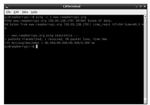
FIGURE 4-2: A successful test of networking on the Raspberry Pi Model B
