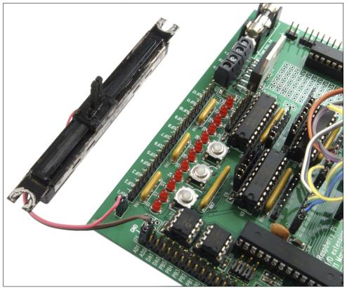
FIGURE 13-10: Connecting a potentiometer to the Gertboard's ADC pins
