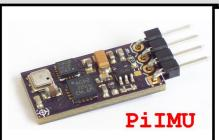
10 DOF Gyro Compass Accelerometer & Altimeter for RPi
