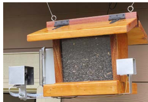
▲ The camera and ultrasonic sensor are set on either side of the area where birds will feed
