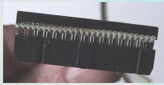
7. Insert the 26 way ribbon into an IDC connector, ensuring the marked wire and the marked pin (wire 1 and pin 1) are lined up.
