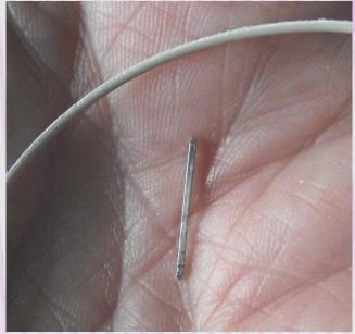
4. Take a length of the seperated wire and carefully remove about 15mm of insulation from each end.
