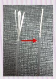
6. Take a pin, put the twisted end of the wire in the centre of the pin and twist the bare wire around the pin toward the end.
