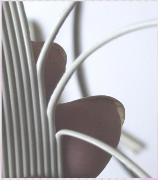
3. Carefully separate out each individual wire, being careful not to rip or break the insulation.
