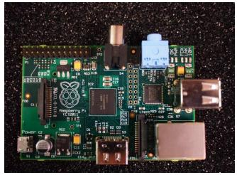
Notably the beta boards were fitted with micro-usb power connectors. This meant that it would be possible to use the commonly found phone chargers to power the boards.
