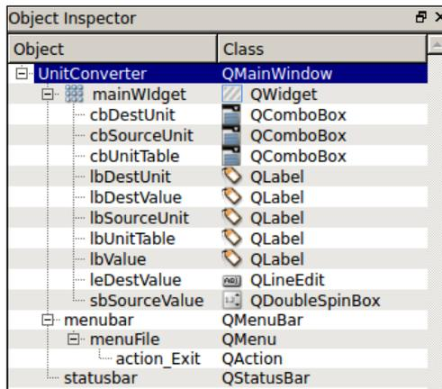
Next, we will disable the **LineEdit** widget that will be used for displaying the result of a unit conversion. This is done by selecting the widget and removing the tick in the **enabled** property in **Property Editor**, as shown in the following screenshot. This is to prevent the user from being able to change the result of the unit conversion.
