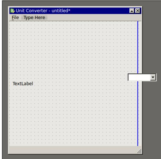
Next, we will add another Label widget underneath the first added one. As before, this is done by dragging it from **Widget Box** and dropping it in the position indicated as follows:
