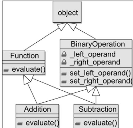
First, we will create the **Function** class that provides an interface for any subclass that inherits from it. Since Python can not explicitly state that a function must be overridden in a subclass, we will have the `evaluate` function raise `NotImplementedError` if it is called on a class that did not override it. This is used to indicate to the code that called the function that an error has occurred, and is done using the `raise` function.
