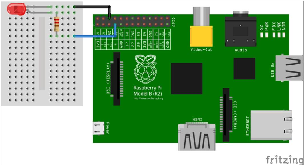
Note that the polarity of the LED is important as electrical current can only flow through it in one direction. The longer lead of the LED is the anode, which should be connected to the resistor, and the shorter lead is the cathode, which should be connected to the ground pin of the Raspberry Pi.
