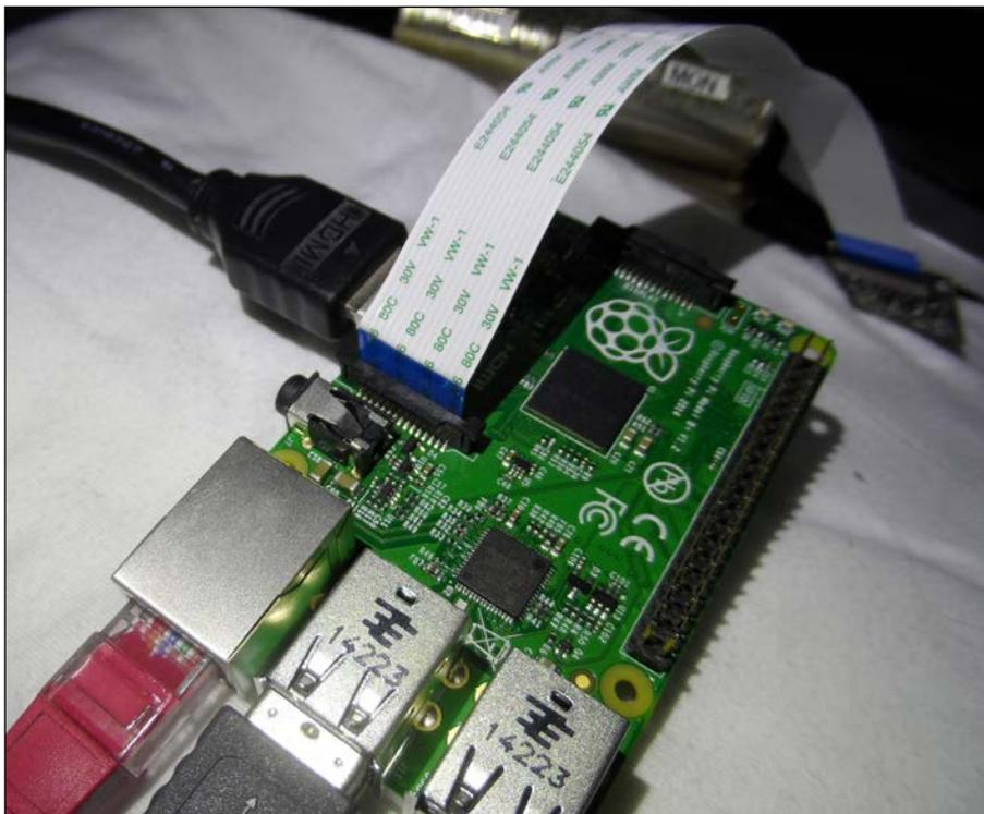
Now that the camera is connected, we will enable it in Raspbian using the `raspi-config` utility.
