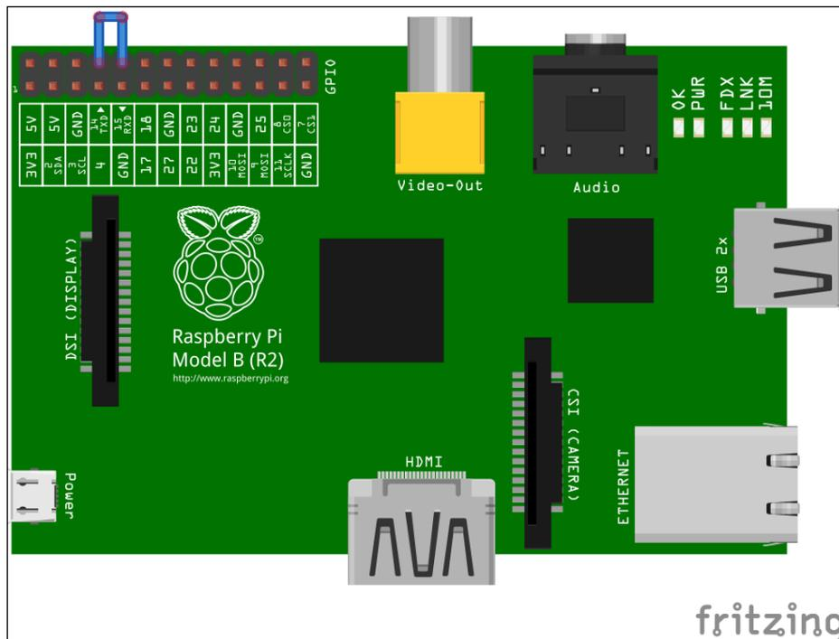
Now, we will use the pySerial library to write a sample script that will send some data to the serial port and read it back. We will save this file as `pyserial_loopback.py`.
