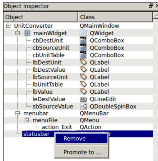
That completes the user interface that we will use for our unit converter application. However, this uses only a small subset of the functionality within the Qt framework for creating the user interfaces.
