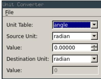
The user interface can now be used to perform unit conversions by selecting a unit table, source, and destination units, and then entering a value in the source value spin box, as shown in the following screenshot:
