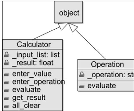
Here each block represents a class, with the second square representing the member variables of the class and the bottom representing the functions.
