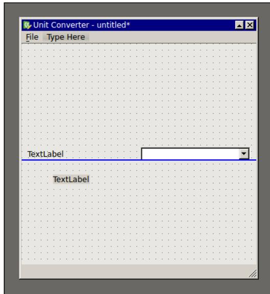
Now, we will add the remaining widgets. This should consist of five Label widgets in the left hand column of the grid layout and two ComboBox widgets, one DoubleSpinBox, another ComboBox, and a LineEdit widget (in that order) in the right hand column of the grid layout, as shown in the following screenshot:
