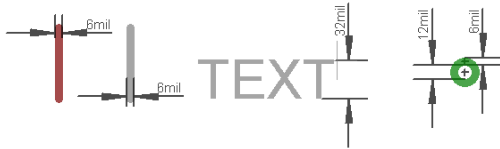
Minimum trace/silkscreen/text/hole size
