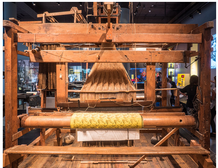
Figure 1. Jacquard loom, one of the first programmable devices
