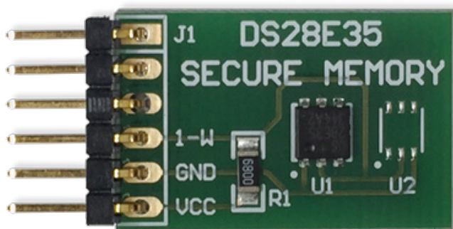
Figure 3. Maxim's DS28E35 DeepCover Secure Authenticator provides crypto-strong authentication security for a variety of applications, including medical sensors, industrial programmable logic controller (PLC) modules, and consumer devices.
