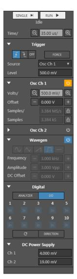
Figure 3-5 Setting up WaveForms Live for our RC circuit exercise.
