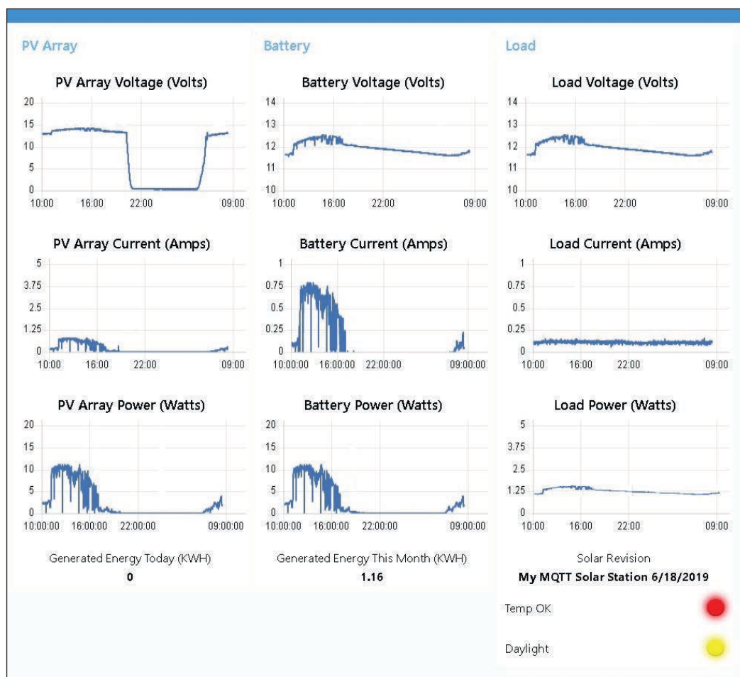
FIGURE 9 The Solar dashboard is one of many that are needed to show all the registers available, but this might be the most informative.
