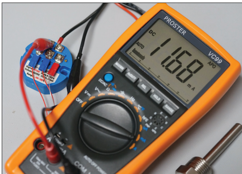
FIGURE 6 Multimeter measuring current from the transmitter before connecting to the receiver
