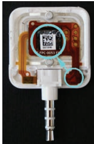
The Square Reader’s encryption chip is located in the bottom right-hand corner instead of on the magnetic head. This drastically reduces the cost of the device.
