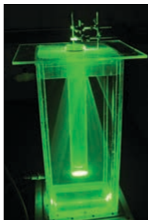
Laser Particle Image Velocimetry (PIV) Tank measuring 2-D flow through a long cylinder
