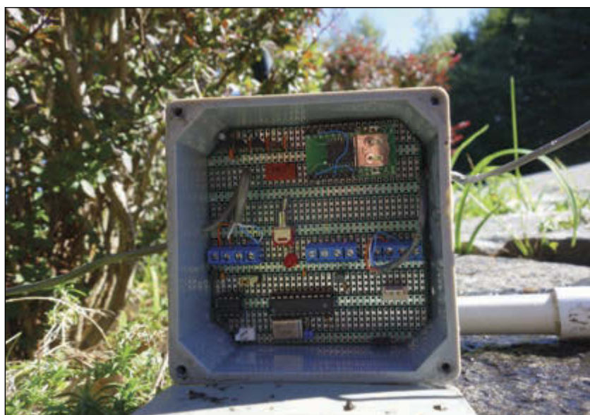
PHOTO 2 The processor (89LPC922), real-time clock (PCF2127), power conditioning, and RS-485 interface chip are visible in this photo. I distribute 12 V over one pair of a two pair RS-485 communication cable and regulate it to 3.3 V and 5 V on the board.
