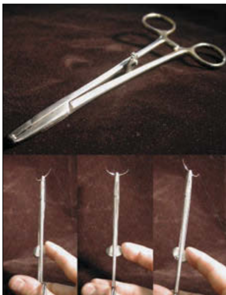
This NeoDriver prototype lets the user change the angle of the suture needle in the jaws of the tool simply by adjusting the angle of a knob; stainless steel wires run from the knob along the left and right sides to rotate a tiny disk embedded in the jaws.
