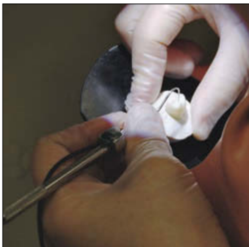
A high-bandwidth MEMS-based accelerometer records the sensations a dentist feels as she probes an extracted human tooth. Feeling these recordings lets dental trainees practice diagnosing dental decay before they treat live patients.
