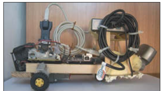
The motors, encoders, and H-bridges. The metal box at the top contains a battery pack, 9-V preregulators, and PI filters. It also acts as a heatsink.
