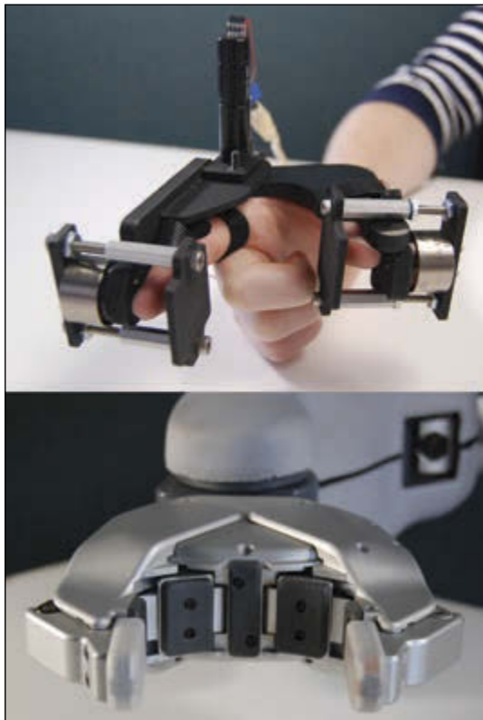
This wearable device allows the user to control the motion of the PR2 robot's hand and also feel what the PR2 is feeling. The haptic feedback is delivered via a geared DC motor and two voice-coil actuators.
