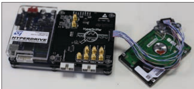
FPGA-BASED "HYPER-SNIFFER"—AN APP-SPECIFIC LOGIC ANALYZER
