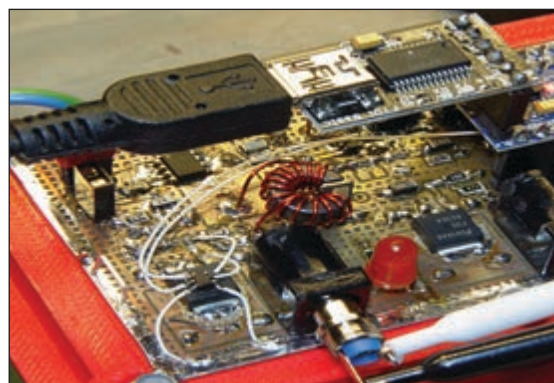
A MAX4544 EPOXIED ON A MOSFET
