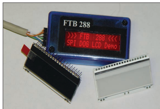
LCD WITH A "COG" DISPLAY AND A BACKLIGHTING MODULE
