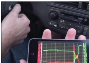
Mooshim Engineering's Mooshimeter displays a car startup transient.
