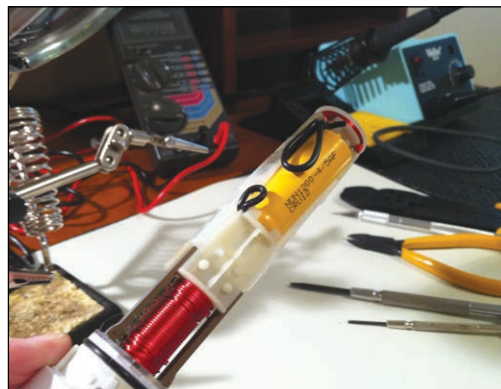
To prolong her toothbrush’s life, Quinn replaced a toothbrush battery with a nickel-cadmium battery and added wires to the old battery’s PCB mount points.
