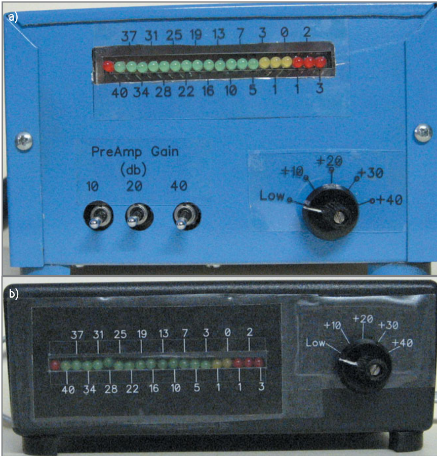
Photo 1a —System 1 is the unit that has both the selectable gain amplifier and a step attenuator. b —System 2 is the unit with just the attenuator.
