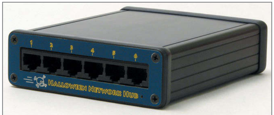
Photo 1—This is the finished network hub design.
