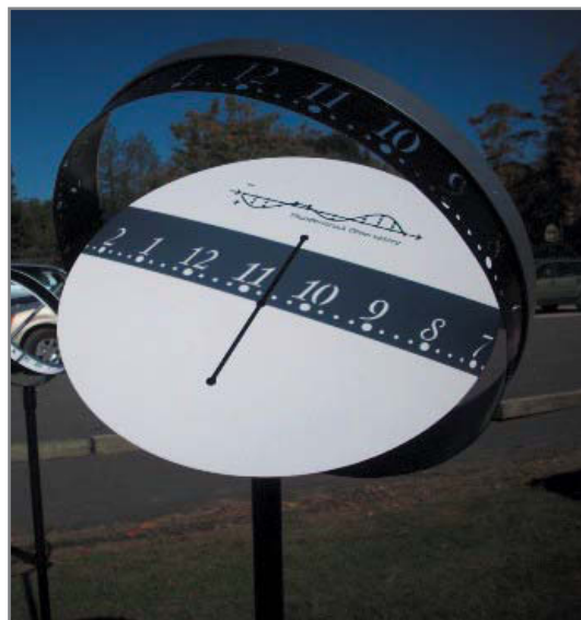
Photo 1 —This sundial uses a shadow mask to display the actual hour glyph on the central area located beneath the ring. As the sun moves, the hour’s glyphs move across the face of the dial.
