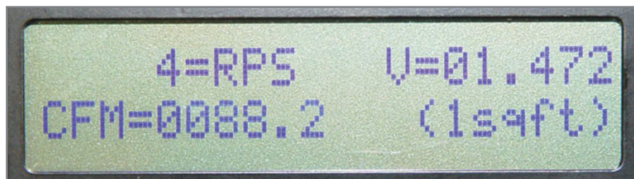
Photo 2 —The LCD displays RPS and velocity. RPS is the Hall effect count/2 (two counts/revolution). The velocity is calculated from a calibration value and the RPS.
