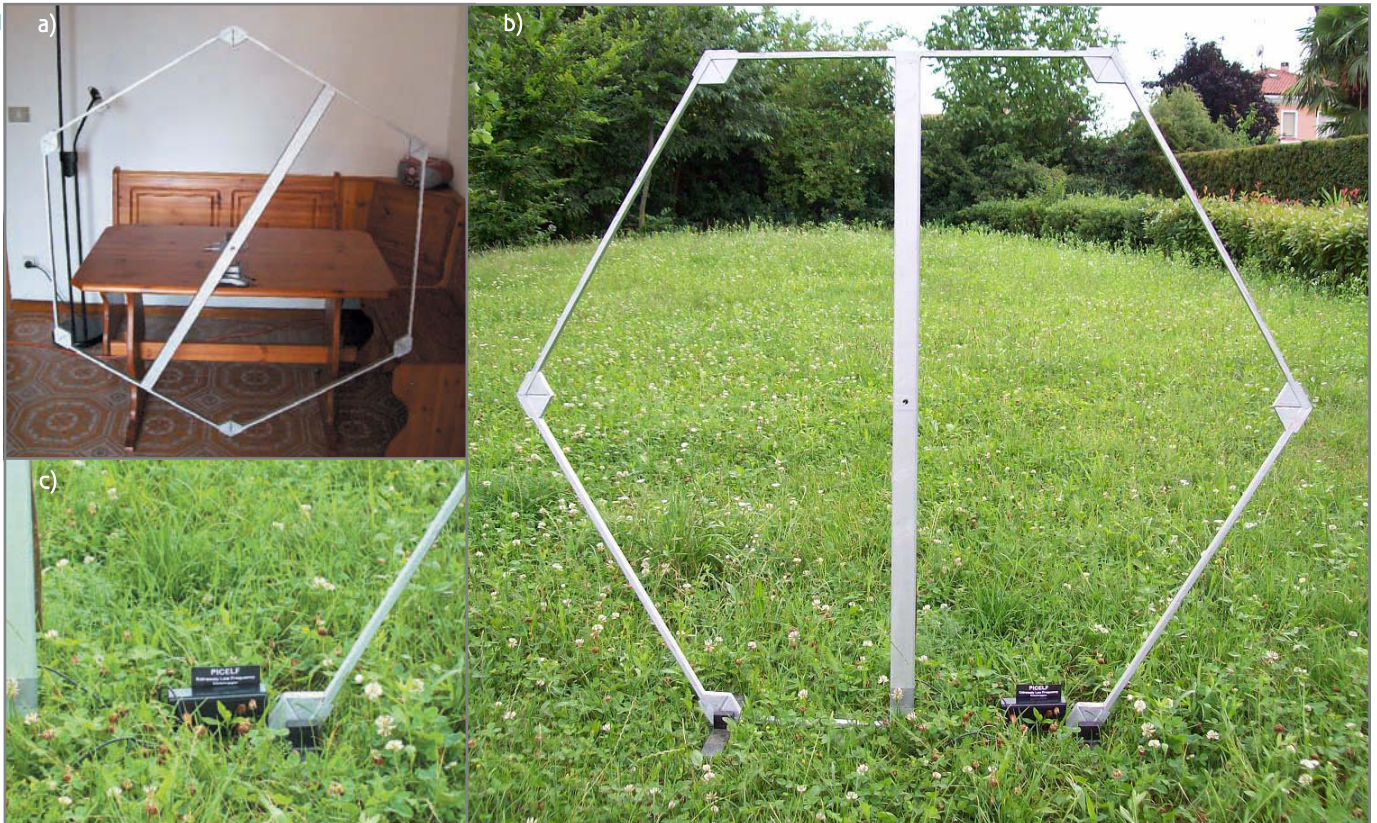
Photo 3a —Here you see the hexagonal loop antenna during wrapping. Notice the hole in the center. It's easy to use for hexagonal rotation. b —This is the datalogger and antenna working in the field—quite literally! c —Take a closer look at the design at the base of the antenna.
