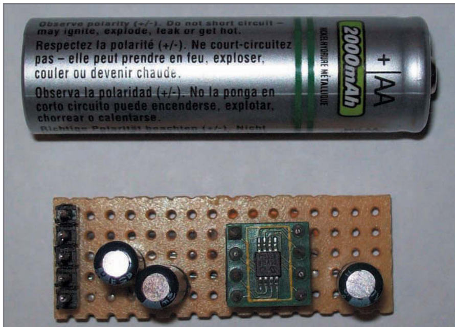
Photo 4 —This is the battery voltage regulator circuit. Note the MCP1253's dimensions with respect to a single AA rechargeable battery.
