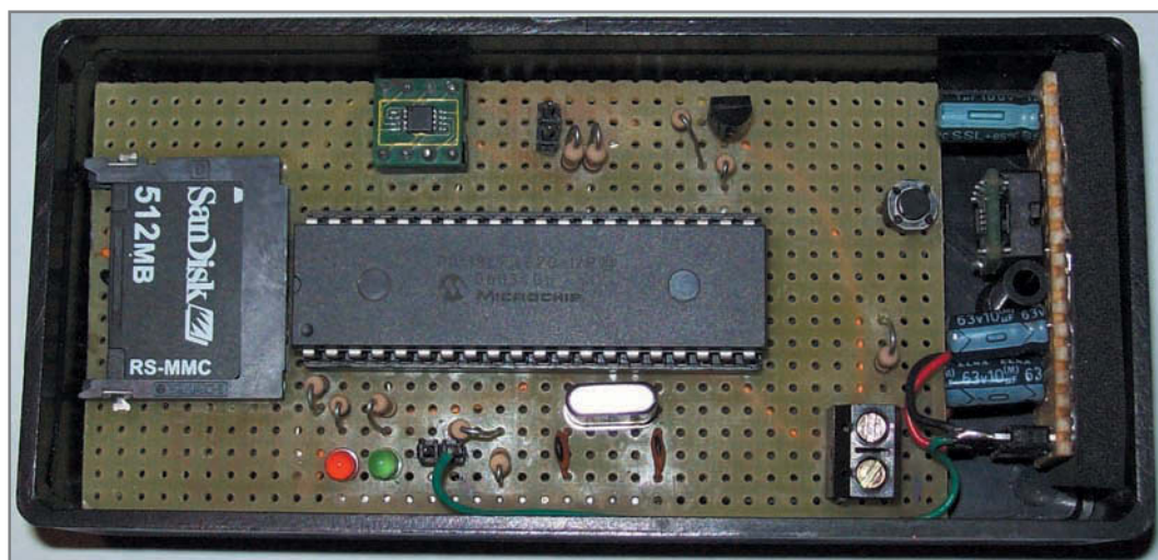
Photo 2 —I created the circuit on two prototype boards. The core is on the left. The battery voltage regulator is on the right.
