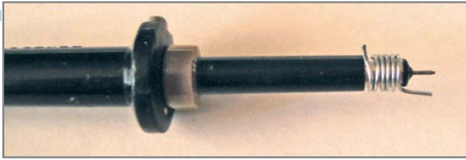
Photo 3 —This is the scope probe. The small ground clip on the end of the scope probe will help reduce the ground lead “antenna effect” picking up magnetic field-coupled noise and other radiated signals.
