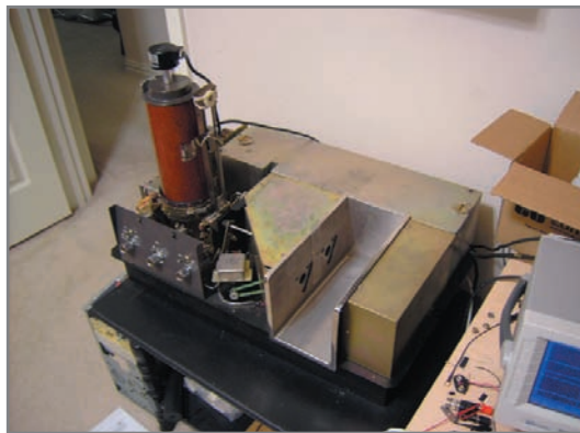
Photo 1 —This 1954 Perkin Elmer 337 spectrophotometer generates infrared radiation and passes it through a chemical sample. Depending on the molecular structure of the sample, it will absorb only at specific wavelengths. The absorption at each wavelength is measured and plotted. The plot is then used to determine the chemical sample.
