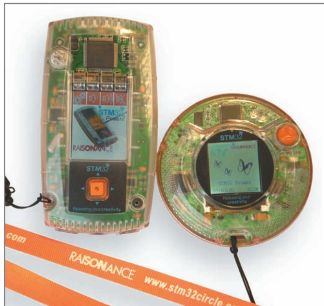
Photo 2 —Take a look at both Primers. The new Primer2 (part number STM3210E-PRIMER) is rectangular. Compared to the original, it has a larger color LCD with touch screen, more flash memory, and more SRAM.
