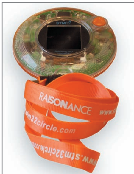
Photo 1 —The STM32 Primer (part number STM3210B-PRIMER) is a self-contained medallion. It includes a neck lanyard, rechargeable batteries, color LCD, sound, a USB interface, a built-in JTAG, and a three-axis accelerometer.
