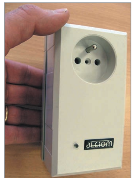
Photo 1 —The PowerSpy is a power analyzer based on a small plug-type measurement system linked through Bluetooth to a PC hosting real-time waveform calculations and a user interface.
