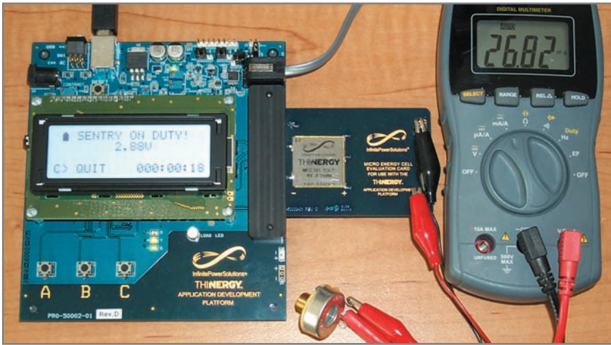
Photo 2 —The MEC lives up to the claims in the datasheet. It delivers tens of milliamps without breaking a sweat—more than enough juice to power-up some pretty fancy silicon.
