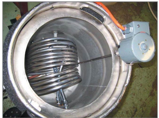
Photo 4 —Take a look at the sparge tank. You can see the heat exchanger, heater, and the sensors. I took this photo after the stir motor was attached (key learning).
