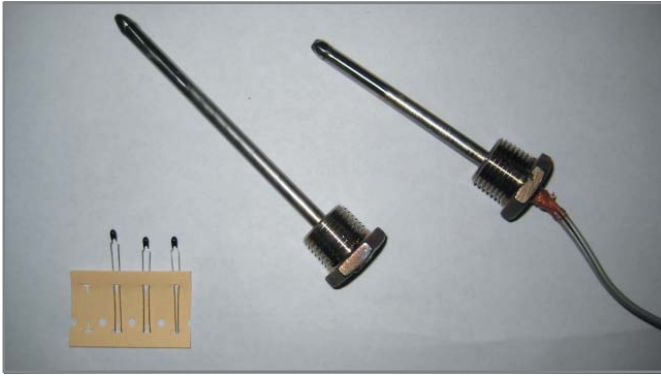
Photo 3 —These thermistor assemblies were made by TIG welding stainless steel tubing to 0.50" threaded and drilled plugs. The thermistors are shown in the bottom-left corner. Wires were soldered along with heat-shrink tubing to form the electrical assembly.
