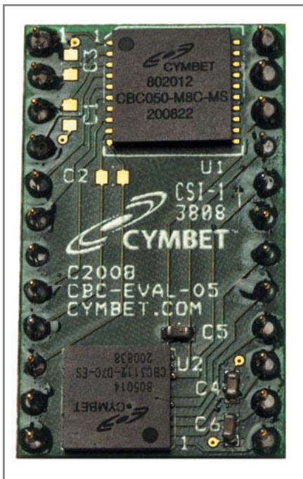
Photo 1 —The CBC-EVAL-05 includes both 50- \mu Ah (CBC3150) and 12- \mu Ah (CBC3112) EnerChips. It's easy to switch between one or the other just by rotating the module.
