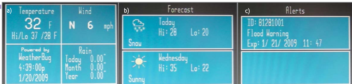
Photo 2a —The Current Conditions screen shows rainfall totals, temperature, and average wind direction and speed. b —The Forecast screen shows the high and low temperatures, as well as the expected conditions for the next two time periods. c —The Alerts screen displays active weather alerts and updates.
