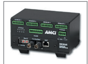
Photo 3 —The Nexus SSI Interface Controller supports up to four SSI devices and has options for ControlNet, DeviceNet, Ethernet IP, and Modbus TCP/IP. Unfortunately, it lacks an LCD. This SSI controller requires a PC to view readings from the position sensor.
