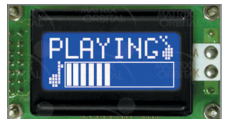
Photo 4 —The LCD0821 has a 2 × 8 line alphanumeric liquid crystal display. It supports both RS-232 and an I 2 C communication interface.
