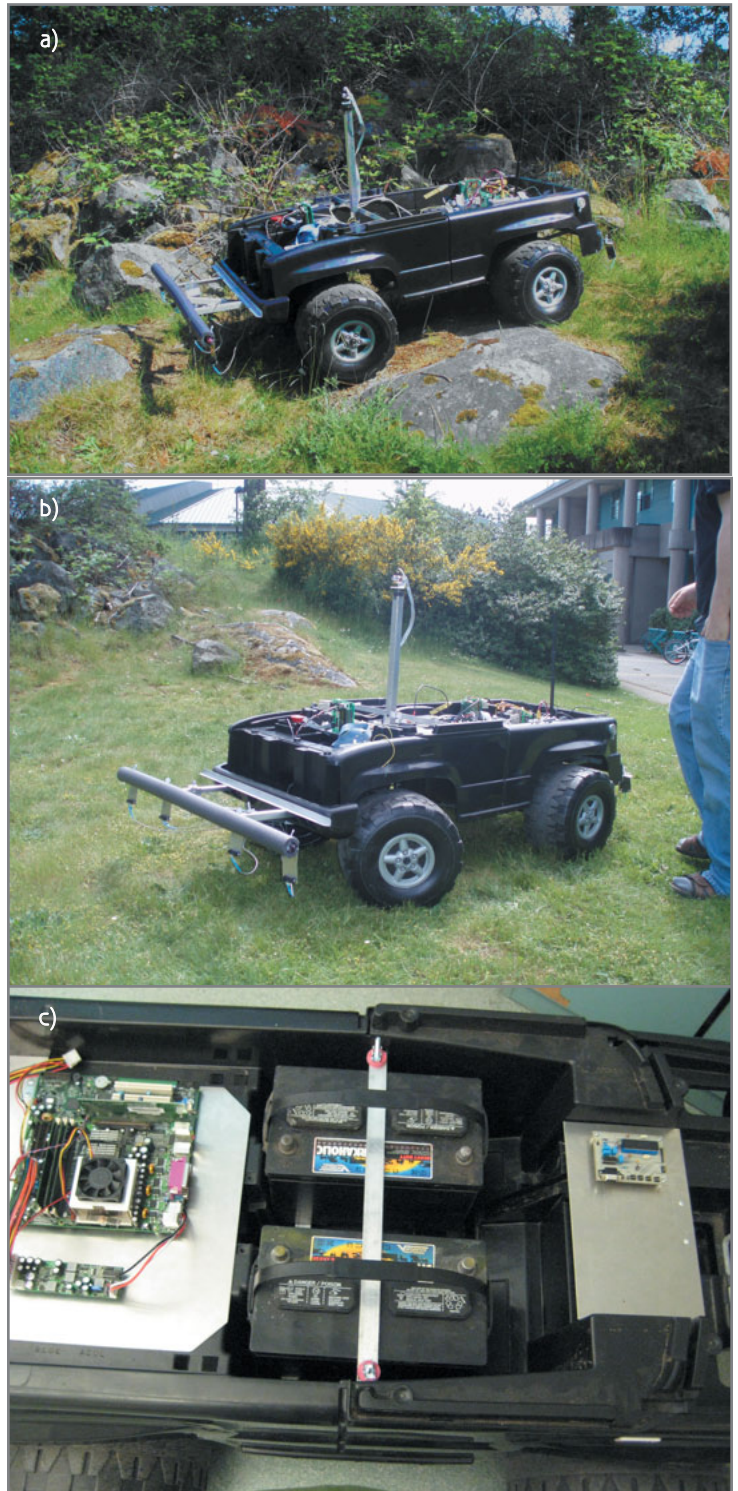
Photo 1a —Take a look at the Interurbanator in action. Here it's traversing fairly rugged terrain. b —IR range sensors enable the vehicle to avoid obstacles like people (seen here) and stationary objects. c —The design features two 12-VDC motors and a simple chassis. Everything fits nicely inside.
