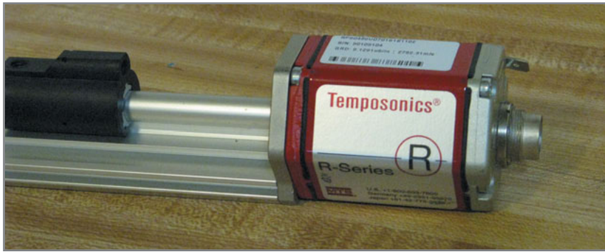
Photo 2 —Unlike other sensors, the Temposonics III R-series linear position sensor can be reprogrammed in the field. Programmable options include: changing the sensor's resolution, output data format and the type of communication interface, synchronous or asynchronous.
