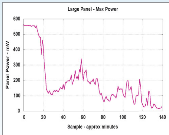
Figure 4—The panel's maximum power output varies dramatically due to clouds, tree shadows, and angle of incidence. Each data point represents slightly more than one minute of elapsed time.
