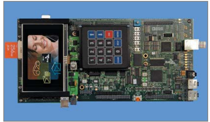
Photo 2 —The BF548 evaluation board has significantly more capabilities than the BF533 evaluation board with many peripheral devices, including a colored touch screen.
