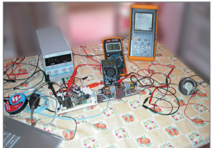
Photo 1 —This test set verifies H-bridge and PID parameters. The motor under test is mechanically joined with a similar motor. This one is loaded on a power variable resistor to easily simulate a variation in mechanical load for the first motor.
