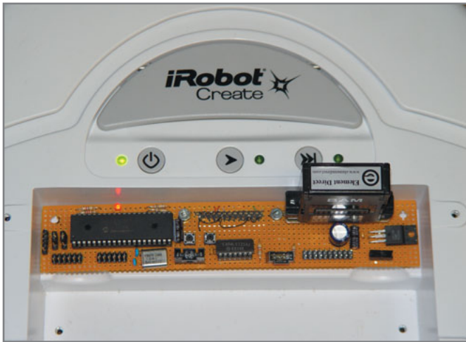
Photo 1 —I built the Create Commander circuit to the same dimensions as the CM. It fits on the cargo bay connector and provides I/O expansion and Bluetooth wireless connectivity.
