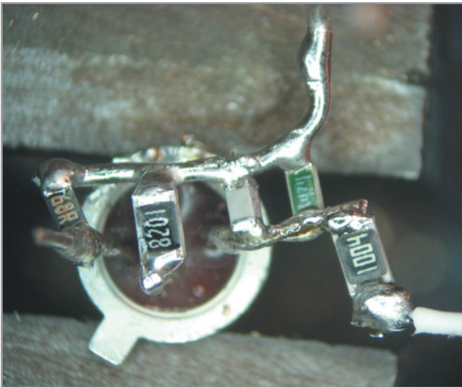
Photo 1 —The flying SMT technique required some patience, but it enabled me to build a compact pulse generator without any specific PCB (thereby minimizing any parasitic inductance or capacitance).
