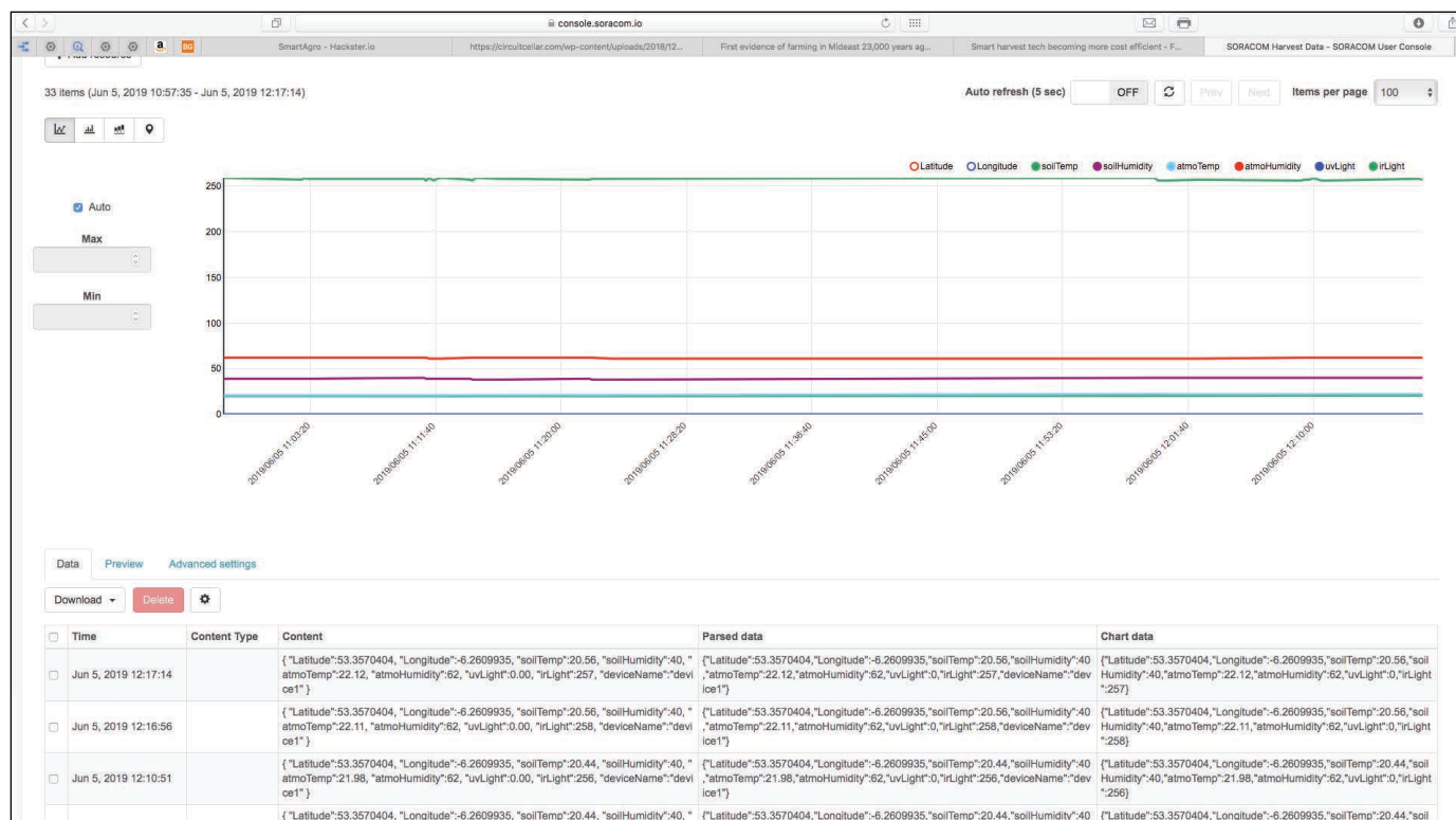
FIGURE 8 The populated graph and table with the JSON data sent by the MKR GSM
