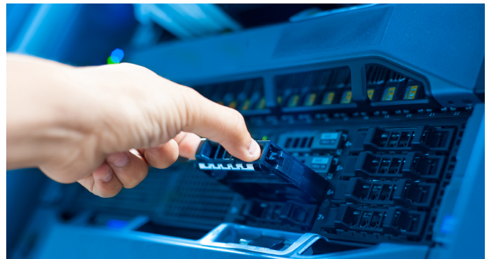
Figure 34. Hot Plug-In Causes Voltage Surges
