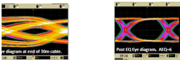
Figure 9. Contrast Between Closed (left) and Open (right) Eye Diagrams
